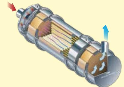
Droplets of Diesel fuel are injected between the filter and an additional decomposition catalyst to reduce  $\text{NO}_2$  levels. A filter monitor controls the injection rate depending on the exhaust gas temperature and the engine speed. This system reduces 99.8% of the number of particulates, 90% of the CO and HC, and  $\text{NO}_2$  is kept at the engine out level.
