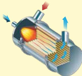
A fuel burner is used to raise the temperature inside the filter to remove the PM. These systems use diesel fuel from the tank and on-board voltage. The regeneration units are mounted on the machine.
