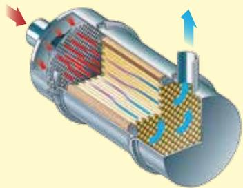
This system uses air to burn the carbon in the filter. An additive in the fuel acts as a catalyst, oxidising the PM trapped in the filter. This additive reduces the temperature at which the carbon will react with the air.
