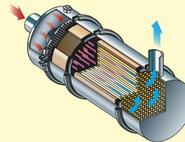
These continuously regenerating systems use a diesel oxidation (DOC) catalyst in front of the filter, which removes carbon monoxide (CO) and hydrocarbons (HC) and oxidises some of the nitric oxide (NO) in the exhaust to nitrogen dioxide (NO<sub>2</sub>). This NO<sub>2</sub> then reacts with the trapped PM, producing NO and carbon dioxide (CO<sub>2</sub>) and cleaning the filter.
