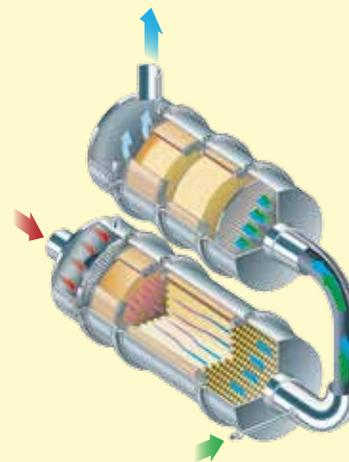
The SCRT® system combines the CRT® system to control CO, HC and PM and a selective catalytic reduction (SCR) catalyst to reduce oxides of nitrogen ( $\text{NO}_x$ ). SCR technology provides the highest  $\text{NO}_x$  reduction available. Johnson Matthey's SCRT® system reduces all four regulated exhaust emissions: CO, HC and PM by over 90% and  $\text{NO}_x$  by over 70%.
