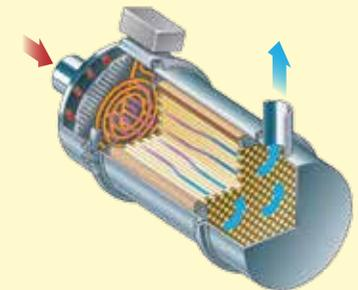
An electrical heater is used to raise the temperature inside the filter to burn away the PM. Air from a small pump is heated to more than 600°C and blown through the filter to remove the carbon. These systems use mains electrical power to regenerate the filter at the end of a shift.
