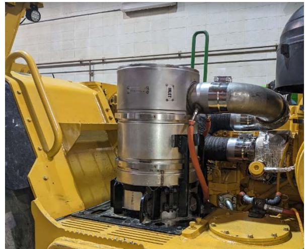
Mining CRT: DOC + DPF + NO 2 DeComp filtration for low NO 2 with superior CO and DPM reduction
